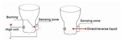
High voltage burn, soaking and flush clog with real time monitor
