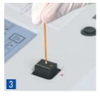
Insert a capillary tube (containing a sample) into the holder.
