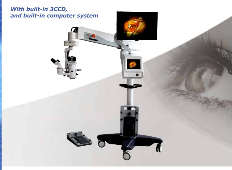
The SOM-4000 operation microscope is a double binocular microscope. The main microscope has zoom magnification system, adapt to different operation by changing the object lens. The assistant microscope has five-step magnifications, it can be locked at 90°to the left or the right of the main scope. Both of the two microscope has the visual angle of eyepiece which can be adjusted from 0° to 180°. The illumination system adopts double lights source meets customers' demand for personalized.
